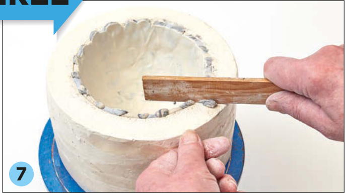
7 ▲ Level the top of the pot using a piece of wooden batten – sit the wood flat on the plaster rim and draw it towards your body in small sections, working around the edge carefully.
