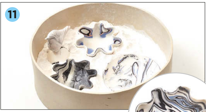
11 If using porcelain, you will find it useful to fire your pieces in a purpose-made clay container, large enough to hold several small pieces at once. Fill the container with alumina to support the pieces as they fire – this will go a long way to preventing the shapes from sagging or distorting. Be aware that this firing method only works for bisque firing or firing up to temperature without glaze. Glazed pieces will need to be fired separately.
