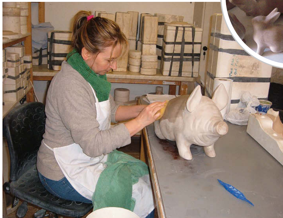
▲ The moulded pieces are fettled and then allowed to dry. (Photo: Griselda Hill Pottery) Inset: Moulded pieces drying ahead of their first firing.
